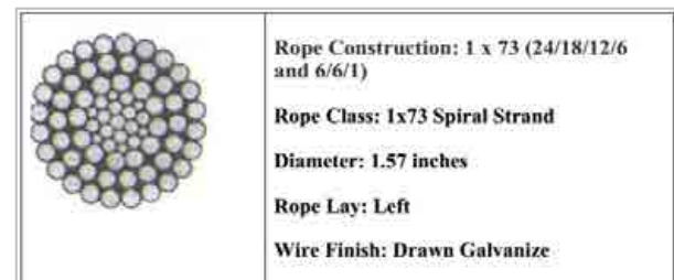
FIGURE 3 – Cable Configuration (Typical)
