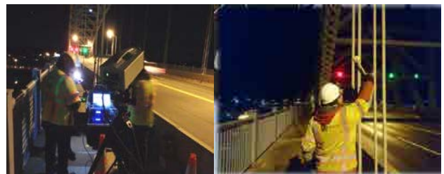
FIGURE 8 – Tension Force Measurement of Suspender Cables
