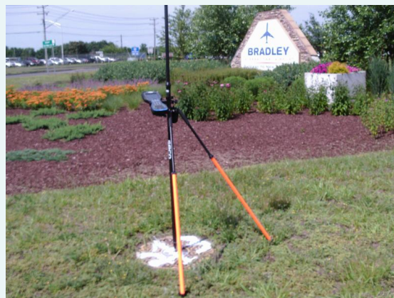
A data collector identifying the location & elevation of a manhole at an entrance to Bradley International Airport
