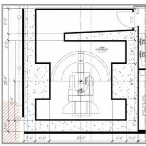
AI has designed a building addition to house a new Linear Accelerator (LINAC) device at the Veterans Administration Medical Center facility in Jamaica Plain, MA. A linear accelerator is the device most frequently used for beam radiation treatments for patients with cancer, and AI is proud to be a part of such an important project.
